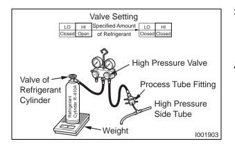
Remove the charging hose (green) from the vacuum pump, and connect it to the refrigerant cylinder
