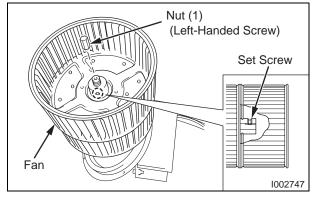
**4)** Take off the four (4) nuts, and then remove the evaporator fan motor together with the motor stay, inlet ring, and fan.
