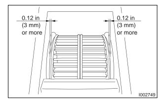
• Install evaporator fan. Allow a clearance of 0.12 in (3 mm) or more on side of the evaporator fan.
