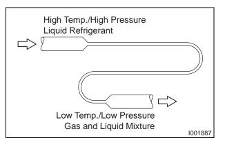
the fixed orifice in the capillary tube. As a result, the temperature and state of the refrigerant becomes low and mist-like, and therefore evaporates easily.
