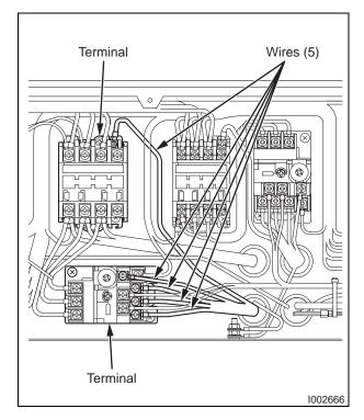
**1)** Disconnect the five (5) wires of the condenser fan motor from the terminals.
