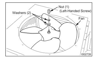
**3)** Take off the nut (left-handed screw) and two (2) washers, and then remove the condenser fan.
