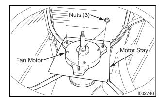
**4)** Take off the three (3) nuts, and then remove the condenser fan motor.
