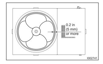
Install condenser fan. Allow a clearance of 0.2 in (5 mm) or more on side of the condenser fan.
