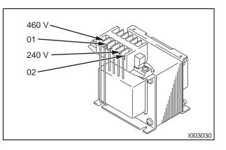
• Terminals 240 V and 02 of the secondary side provide 215 V power source.
