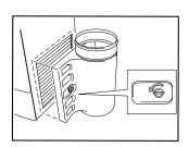
4) Turn the latch of the Air Plenum counterclockwise until it stops. Place the Air Plenum over the condenser openings and align the hinge/bracket assembly mounting holes with the respective screw holes on the back of the unit.
