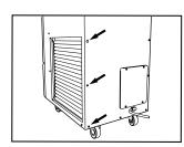
3) Temporairly remove the three (3) screws from the rear panel of the unit.
