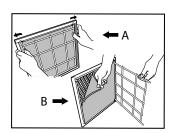
2) Remove the filter elements from the filter frames by pressing outward on the re-tainer at the indicated points (A), then, opening the retainer (B). (Save the filter frames for future use).
