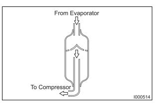
of gravity, causing the refrigerant to accumulate at the bottom of the vessel. As a result, the compressor is protected from possible damage caused by liquid refrigerant intake.
