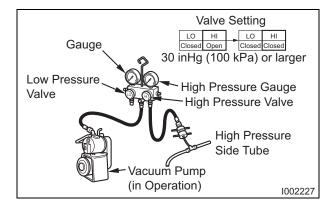
Close the valve of the refrigerant cylinder. Then remove the charging hose (green) from the refrigerant cylinder, and connect it to the refrigerant recovery machine.
