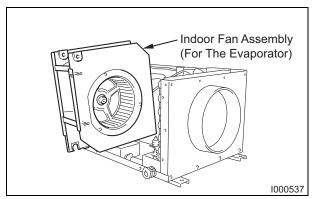
Disconnect the three connectors (two white, twopin connectors; one white, three-pin connector), and then take out the two (2) screws and the two (2) nuts.
