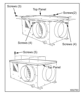
**1)** Take out the four (4) screws, and then remove the service panel.
