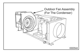
2) Disconnect the motor connector (white, six-pin) from circuit board CN22, and remove the indoor fan assembly (for the condenser).
