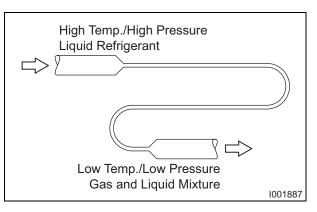
is sprayed out through the fixed orifice in the capillary tube. As a result, the temperature and state of the refrigerant becomes low and mist-like respectively, causing it to evaporate easily.
